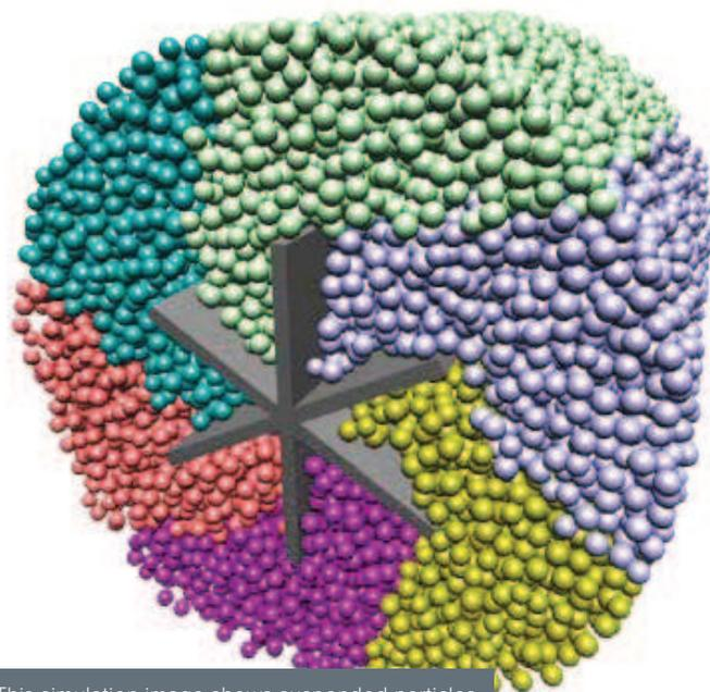
This simulation image shows suspended particles in a rheometer for NIST's proposed mortar SRM. The spheres, which are color coded by their starting location in the rheometer, are suspended in a cement paste with properties derived from NIST's cement paste SRM.
